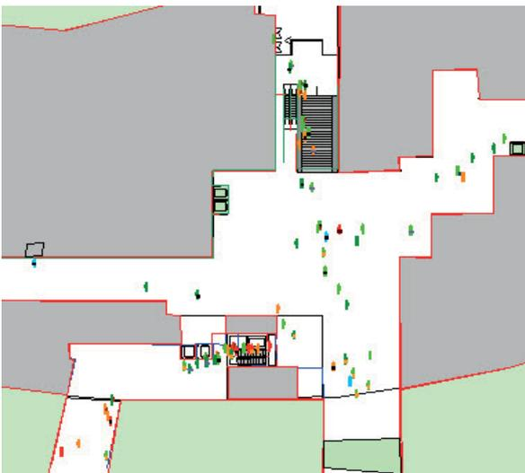
In urban settings, the peak hours in the morning and in the evening are the most stressed situations for any proposed design. Accordingly, the simulation time frame was set to these hours. The simulation results revealed some hot spots and bottlenecks of high people density and waiting times during peak hours. This potentially would endanger the comfortable and safe
